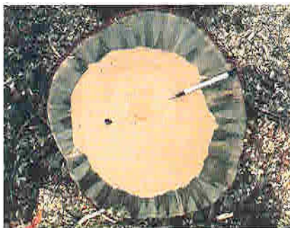
Figure 4 —Sapwood has been discolored by blue-staining fungi; heartwood is not stained.
